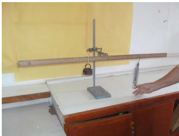
Figure 11.7.2: Experimenting with first order levers
