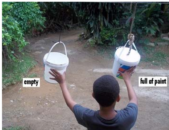
Figure 9.1.7: Two identical containers of different masses used to investigate inertia
