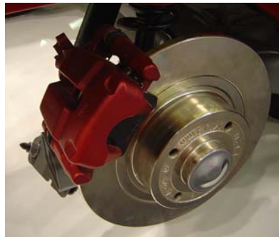
Figure 9.2.2: Hydraulic disc brake
