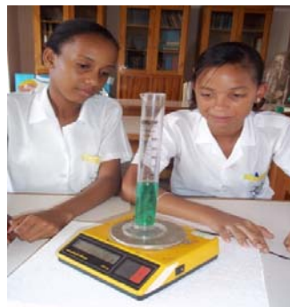
Figure 5.3.3: Two girls measuring the mass of a cylinder containing a liquid
