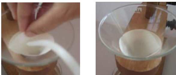
Figure 2.4.1: Procedures for folding the filter paper
