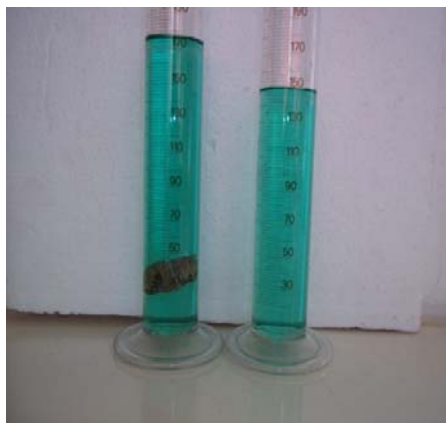
Figure 5.3.2: Apparatus for measuring the volume of an irregular solid
