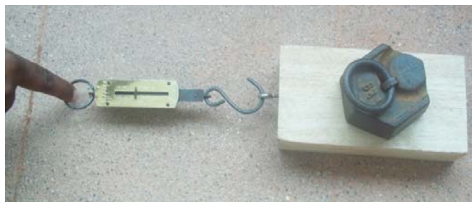
Figure 9.2.1: Set up to investigate frictional force
