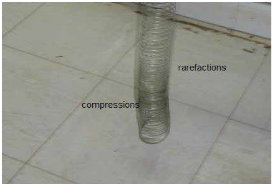
Figure 5b (i): A slinky spring illustrating longitudinal waves. Photo taken by LDTC.
