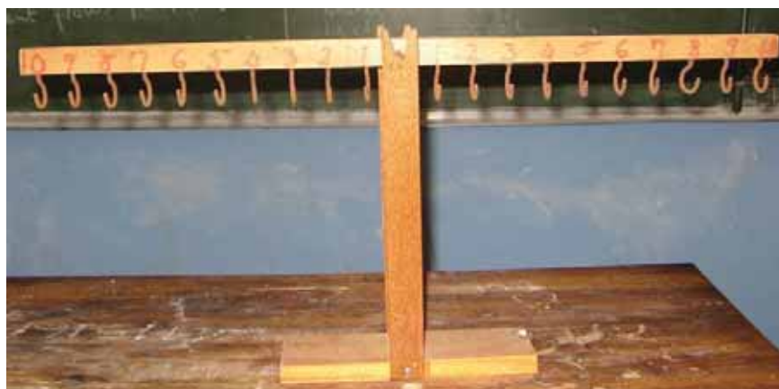
Figure 8: A ruler at equilibrium. Photo taken at the Lesotho College of Education Chemistry Laboratory, 2010.
