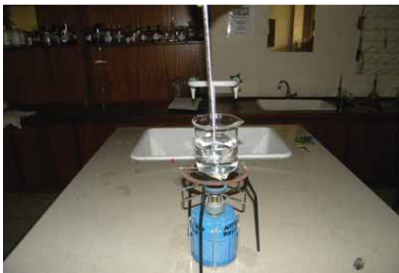
Figure 7: Apparatus for heating water. Photo by Molise Nhlapo at Lesotho College of Education Chemistry Laboratory.
