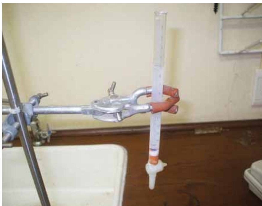
Figure 19: Burette. Photo taken by Molise Nhlapo at the Lesotho College of Education Chemistry Laboratory, 2010.
