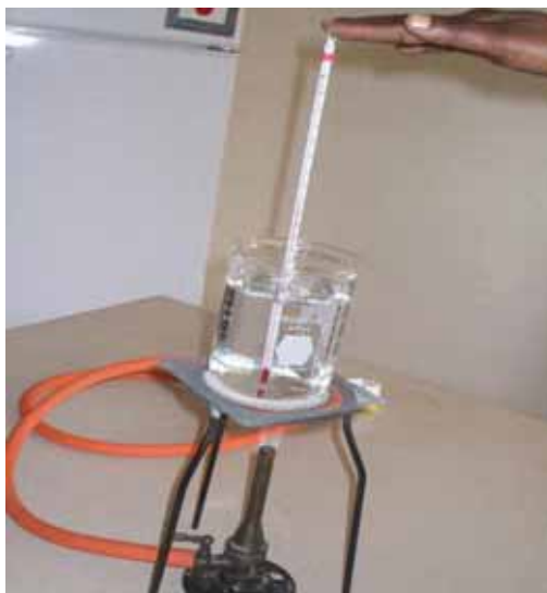
Figure 7: Incorrect measurement of temperature. Photo by Molise Nhlapo at the Lesotho College of Education Chemistry Laboratory, 2010.
