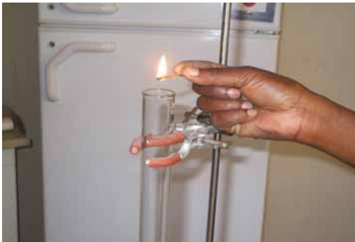
Figure 34: Burning splint placed in hydrogen gas. Photo taken by Molise Nhlapo at Lesotho College of Education Chemistry Laboratory, 2010.
