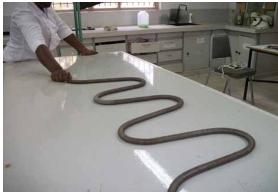
Figure 5(c): A spring illustrating transverse waves. Photo taken by LDTC.
