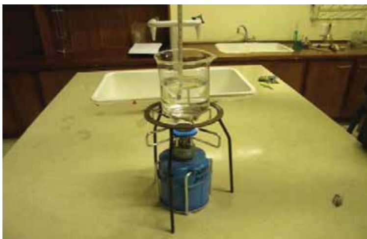
Figure 6: Correct way of measuring temperature of liquids. Photo by Molise Nhlapo at the Lesotho College of Education Chemistry Laboratory, 2010.
