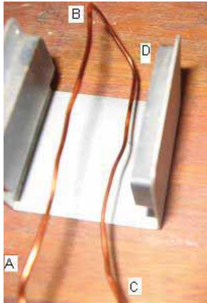
Figure 11(b): Simple AC generator. Photo taken by LDTC.
