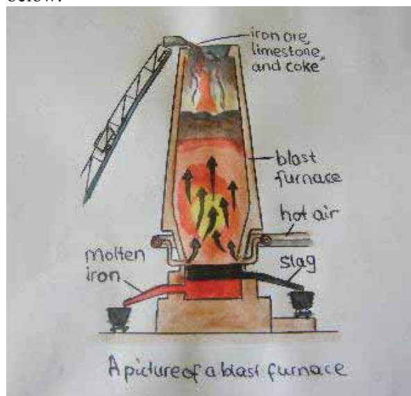
Figure 12: A picture of a blast furnace. Hand drawn by graphic designer at LDTC.
