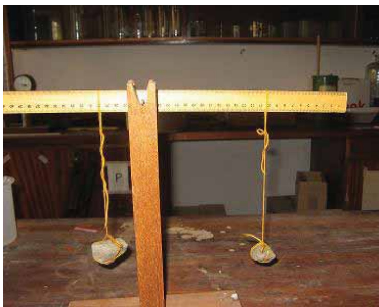
Figure 4: A smaller stone 5 cm from the pivot and larger stone 14.7 cm from the pivot suspended on either side of the ruler. Photo taken at the Lesotho College of Education Chemistry Laboratory, 2010.
